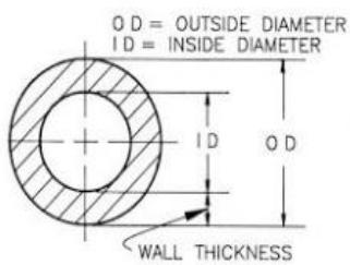
Special terms are used to describe the circular dimensions of the pipe. The inside diameter of pipes is the width of the inner part. The outside diameter of pipes is the actual diameter of the pipe, taking into account the wall thickness.
