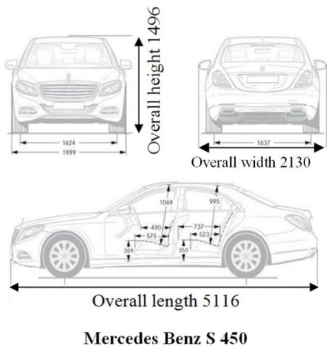
Depth is a linear dimension that defines the distance from the front of an object to its back.
