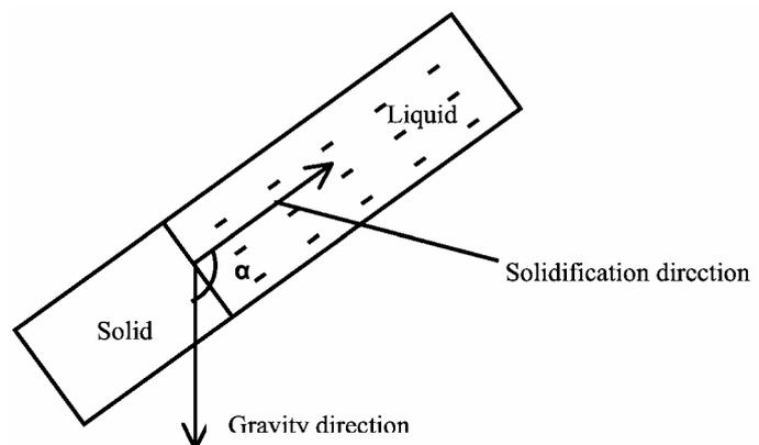
Fig. 1. Schematic of solidification direction  $\alpha=0\sim 180^\circ$
