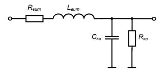
Fig. 1. Equivalent circuit of an elementary coil
