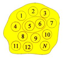
Fig. 2. Arrangement structure of conductors of the coil in a slot of the 4A100S2U3 engine for a part of slot section
