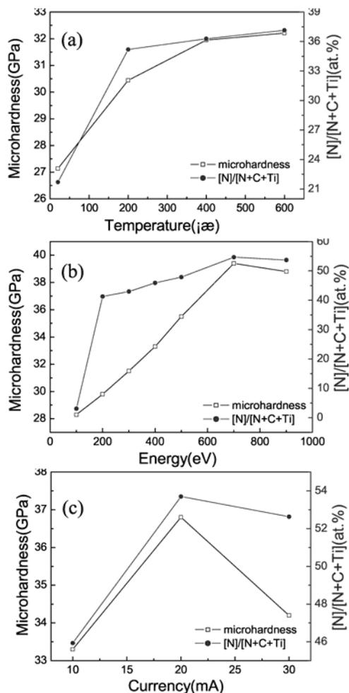
Fig.2. The microhardness and the N concentrations of  $CN_x/TiN_y$  multilayers
