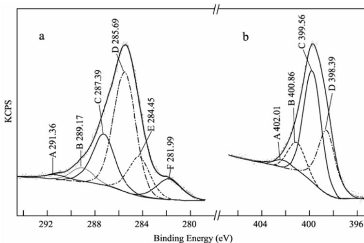
Fig. 1. XPS spectra of the  $CN_x$  layer in  $CN_x/TiN_y$  multilayers
