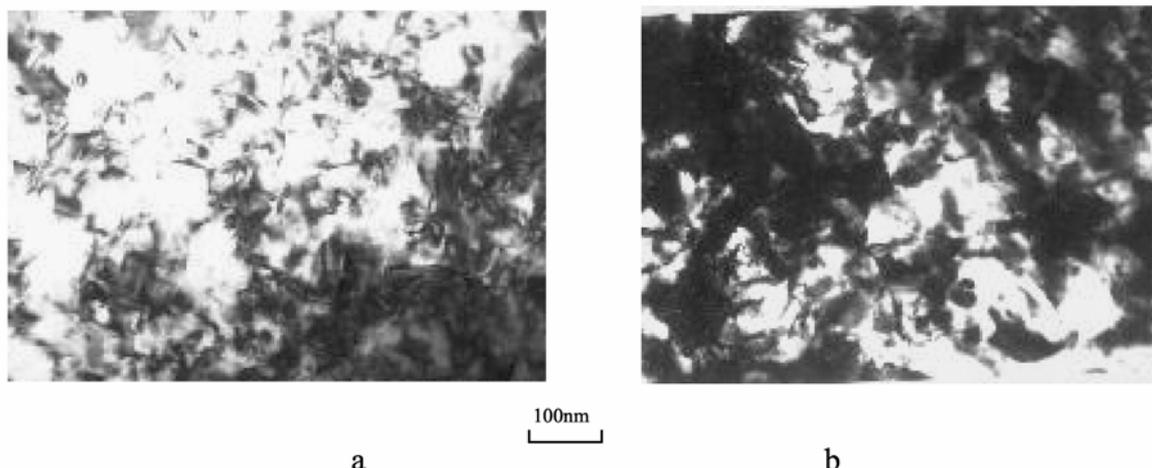
Fig.2. TEM images of recrystallized microstructures in 15CDV6 (a) and in Q235 (b) and (c) 75% reduction, at 580°C for 16h. (b) 93% reduction, at 300°C for 1h
