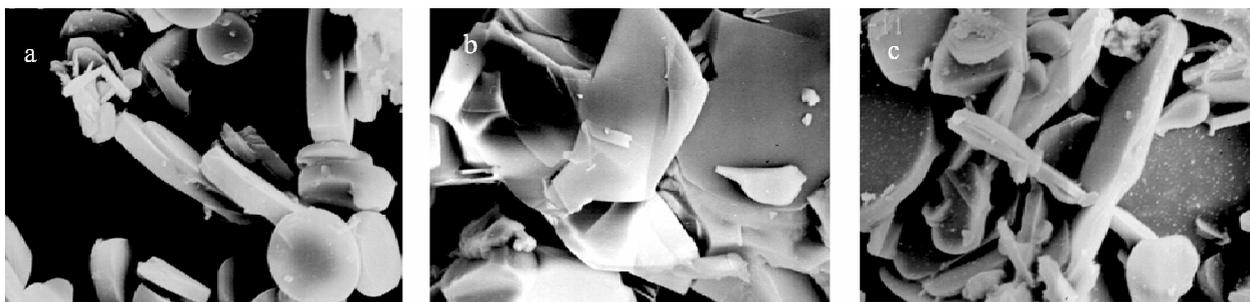
Fig. 1. Morphologies of  $B_2CN$  crystals synthesized by turbostratic  $B_2CN$  precursor and (a) Ni, (b) Fe, (c)  $Ca_3B_2N_4$  catalysts after HPHT treatment at 5.5GPa, 1600°C for 15 min
