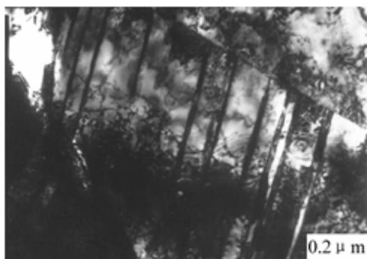
Fig.2. TEM micrograph and diffraction spots of  $\alpha'$ -Martensite
